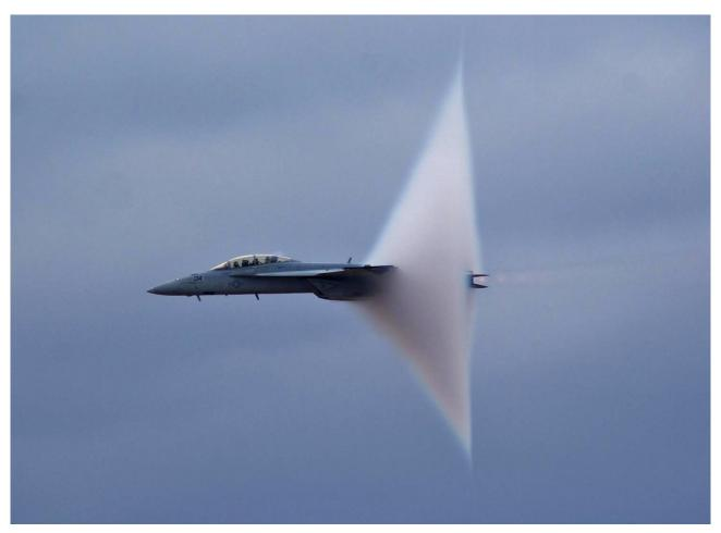
Fig 33 - F18-Hornet travelling supersonic around which a vapour cone has formed. The air surrounding the jet crosses over from hyperbolic, or supersonic, irrotational flow to subsonic and thus elliptic irrotational flow. The parabolic straight line is seen in the vapour cone.
